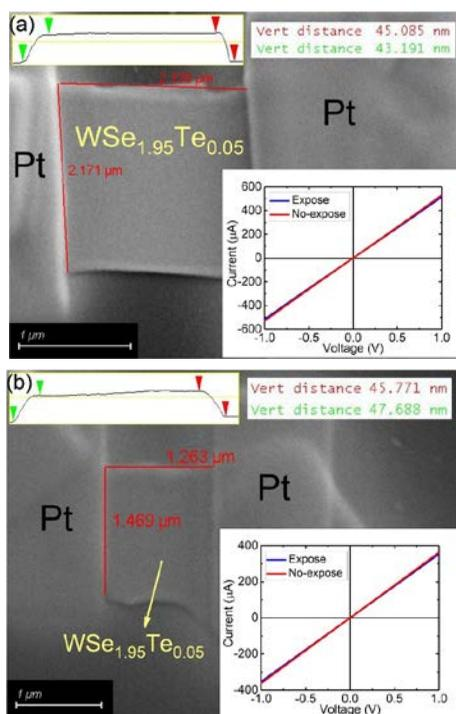
The SEM image of two WSe<sub>1.95</sub>Te<sub>0.05</sub> nanosheets. Two Pt contacts are deposited on each WSe<sub>1.95</sub>Te<sub>0.05</sub> nanosheet. The thickness is 45.0 and 46.7 nm for sample 1 and sample 2, respectively. The linear current-voltage dependence supports the contacts between Pt and WSe<sub>1.95</sub>Te<sub>0.05</sub> nanosheet are ohmic contact.
