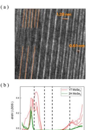
• (a) The HRTEM of the MoSe1.8Te0.2. The lattice distance of 2H structure is 1.28 nm and the lattice distance of 1T structure 0.61 nm.
