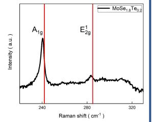
• The Raman spectrum of the MoSe1.8Te0.2. The peak position is lower than the database of MoSe2, the red line. This originates from the replacement of Te atoms.
